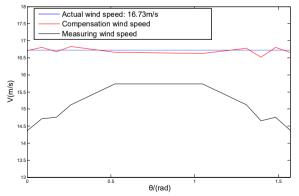
Fig. 6. Comparison before and after measurement of wind speed compensation
