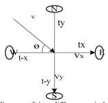
Fig. 1. Schematic diagram of time difference wind speed measurement
