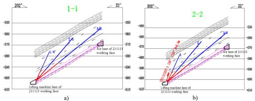
Fig. 11. Layout profile of blast hole
