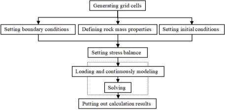
Fig. 2. Framework of FLAC3D calculation
