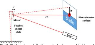
Fig. 3. The laser beam deflection method scheme used in this work
