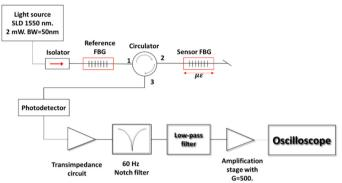
Fig. 4. Experimental setup of the accelerometer
