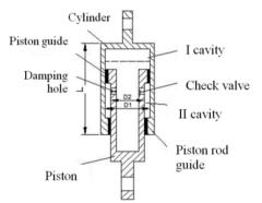
Fig. 2. Front suspension cylinder internal structure
