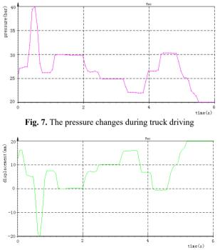
Fig. 8. The displacement changes during truck driving
