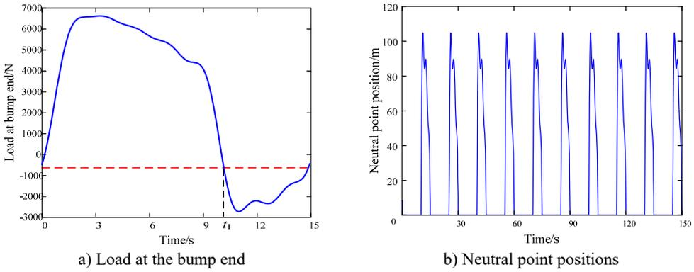
**Fig. 3.** The curve of pump load and the neutral point position with time
