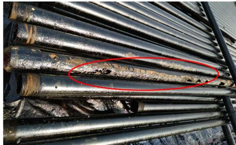
c) The tubing worn out in no. X5 well
