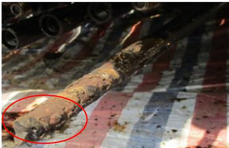
a) The 67th rod worn off in no. X2 well
