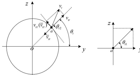
Fig. 2. Velocity change during the collision
