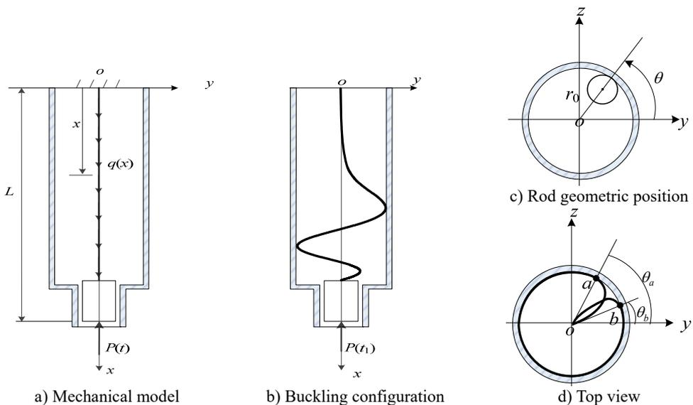
Fig. 1. Transverse bending mechanics model of sucker rod
