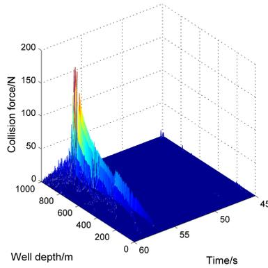
**Fig. 5.** The local curve of collision force with well depth and time (45-60 s)
