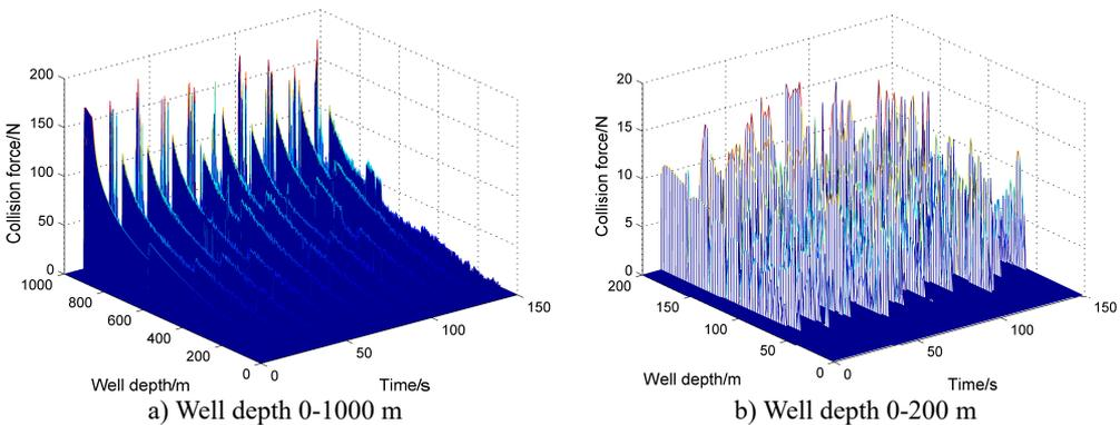
**Fig. 4.** The curve of collision force with the well depth and time
