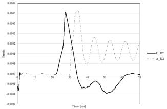
Fig. 8. Comparison of measured and predicted strain for longitudinal reinforcement (TNT 100 kg)
