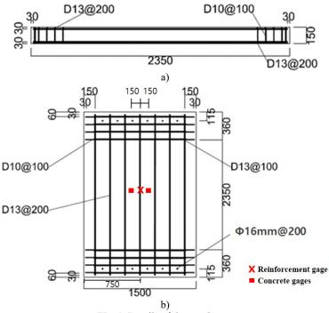
Fig. 1. Details of the specimens
