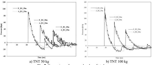
Fig. 7. Comparison of measured and predicted pressure
