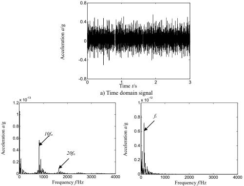
b) Hilbert envelope spectrum of reconstruction signal's slice signal-cyclic frequency equal to outer ring twice characteristic frequency-based on d4 characteristic frequency-based on a4
