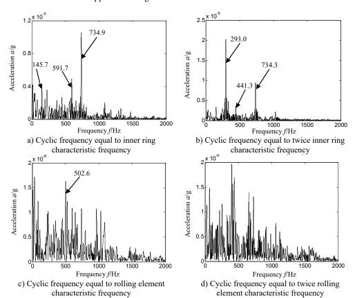
Fig. 7. Hilbert envelope spectrum of original signal's slice signal on different cyclic frequency position-sensor installation on vertical upper of bearing chock
