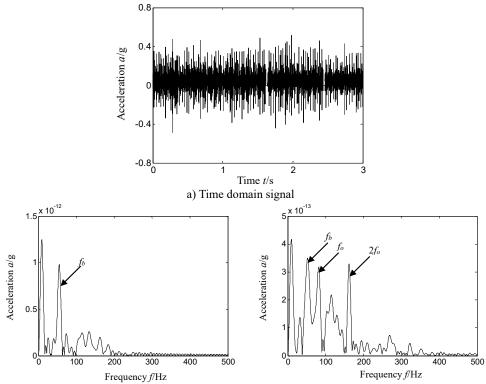
b) Hilbert envelope spectrum of reconstruction signal's slice signal-cyclic frequency equal to rolling signal's slice signal-cyclic frequency equal to outer element characteristic frequency-based on a4
