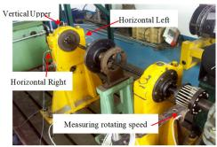
Fig. 1. Aero-engine rotor-rolling bearing experiment rig
