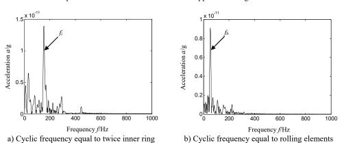
characteristic frequency-based on d4 characteristic frequency-based on a4
