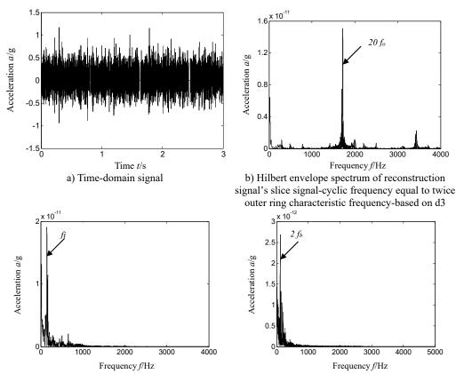
c) Hilbert envelope spectrum of reconstruction signal's slice signal-cyclic frequency equal to inner ring characteristic frequency-based on d3
