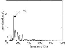
characteristic frequency-based on d4 Fig. 10. Hilbert envelope spectrum of reconstruction signal's slice signal on different cyclic frequency position-sensor installation on horizontal right of bearing chock
