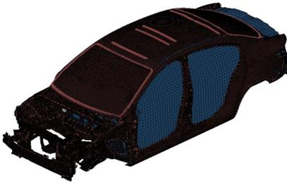
Fig. 4. The FE model of the structure and the acoustic cavity
