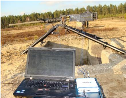
**Fig. 4.** Recoil force measurement equipment
