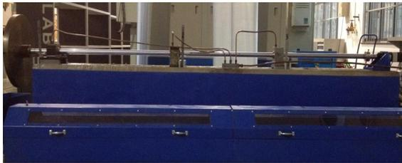
**Fig. 16.** A three-support shaft test rig
