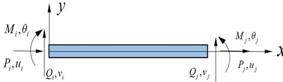
**Fig. 2.** Two nodes element BEAM188 model
