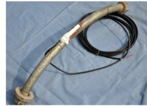
b) Strain gauge on bolt
