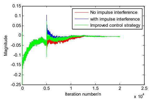
**Fig. 4.** Variation of filter coefficients with iteration
