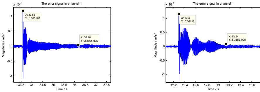
**Fig. 7.** Vibration of the error measuring point after the impulse interference
