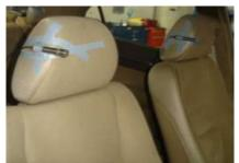
Fig. 1. Microphone positions for testing the interior noise
