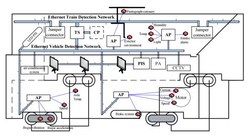
Figure 1. The train security detection network architecture.
