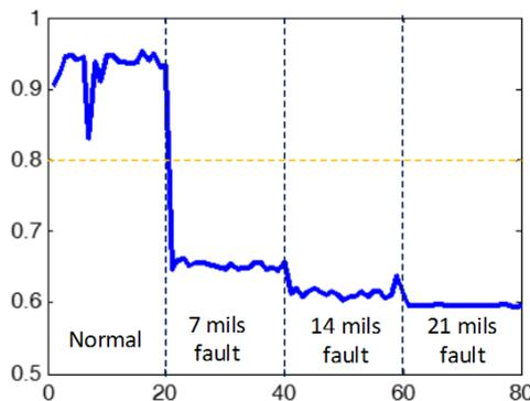
**Figure 3.** CV of different bearings.
