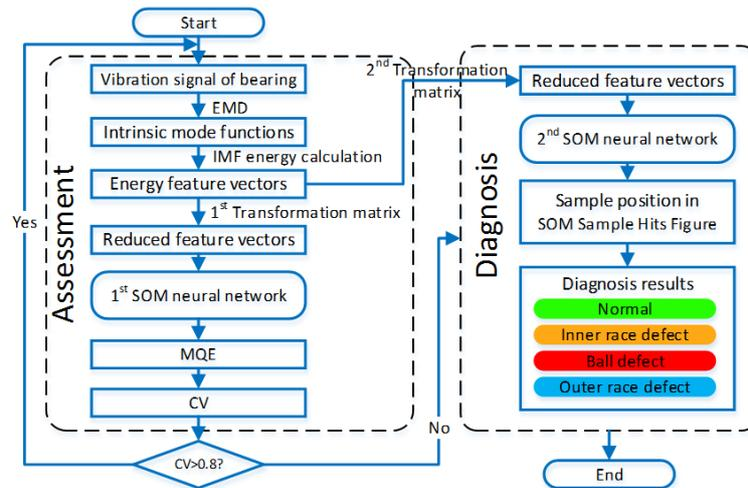
**Figure 1.** Performance degradation assessment and fault diagnosis based on EMD and PCA-SOM.
