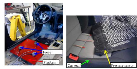
Fig. 7. Load cells (GTM)
