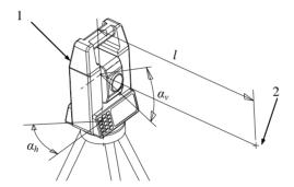
Fig. 1. Point position (coordinates) determination principle by measuring geodetic instrument: l – geodetic instrument (tacheometer), 2 – point which coordinates had to be determined
