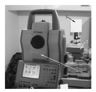
**Fig. 5.** Measurement equipment arrangement for testing of suggested calibration method: *1* – scanning instrument (tacheometer), *2* – turn table, *3* – calibration plate
