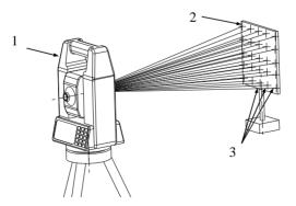
Fig. 2. Mesuring of point cloud of plate surface: 1 – geodetic angle instrument (tacheometer), 2 – measuring plate, 3 – determined points
