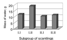
**Fig. 8.** The average water quantity in scantlings: I.I - across and along the fiber, without vibration application, I.II - with vibration application, II.I - across the fiber, without vibration application, II.II - with vibration application
