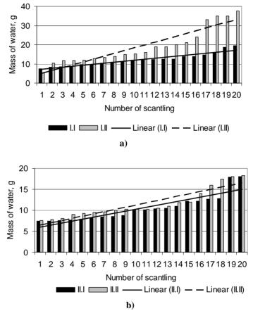
Fig. 7. The comparison of water quantities contained in scantlings: (a) – along and across the fiber; (b) – across the fiber; I.I and II.I – scantlings without vibration application, I.II and II.II – scantlings with vibration application
