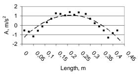
Fig. 4. The mode shape of the scantling vibrating in water
