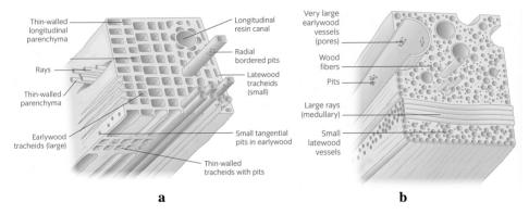
Fig. 2. The macrostructure scheme for coniferous (a) and deciduous (b) wood [10]
